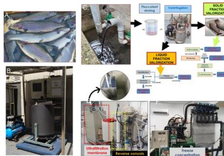
**Fig. 2:** A. Rainbow Trout from Caviar Pirinea SLU; B. Biodrying pilot unit for the valorization of fish sludge and dead fish set in BETA. C. Fish Sludge from the processing plant. D. Dead fish as co-substrate. E. Mechanical process and osmosis. and F. Freeze concentrator
