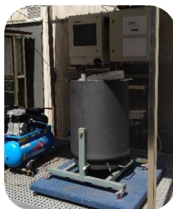
**Figure 1:** Biodrying reactor.
