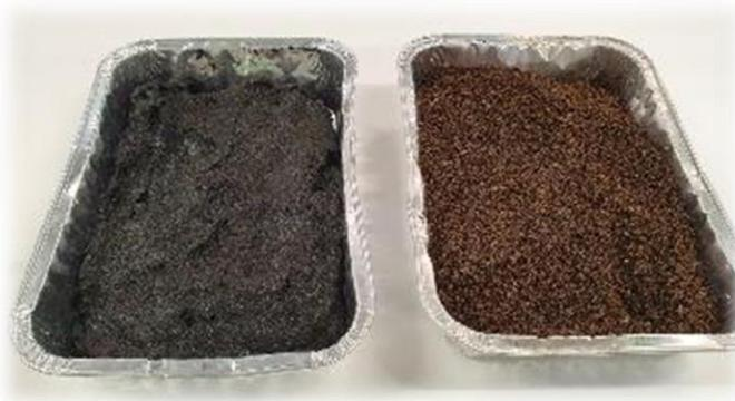
**Figure 2:** Raw wastewater solid fraction (left) and biodried product (right).
