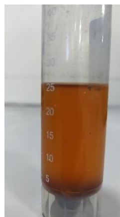
Fig. 3: Oil separated from broken, refrigerated viscera. FFA (Free Fatty Acid): 19 % Peroxides: 9,8 meqO 2 /kg
