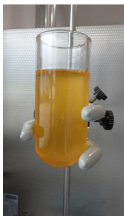
Fig 2: Oil separated from whole, refrigerated viscera. FFA (Free Fatty Acid): 2.7%. Peroxides: 3.5 meqO 2 /kg
