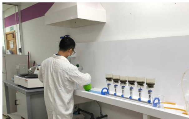
Fig 2: Vacuum filtration can achieve needed TSS in pre-concentration small scale for shipping, but is labour and time intensive
