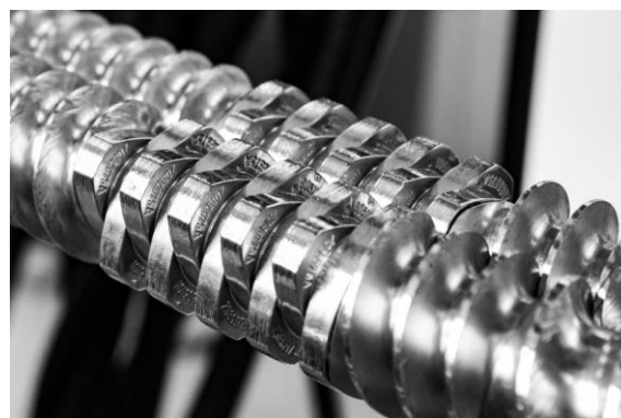
Fig 2: Example of extrusion screw profile
