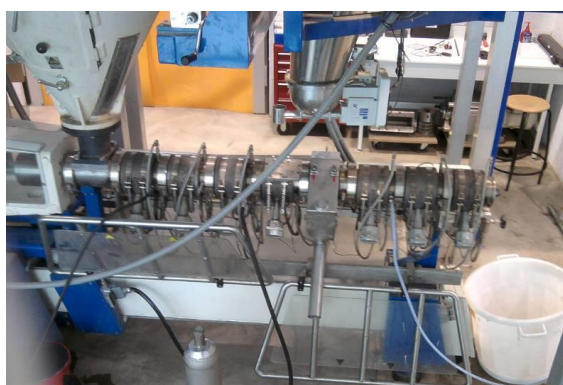
Fig 1: Evolum HT53 (Clextal) twin screw extruder
