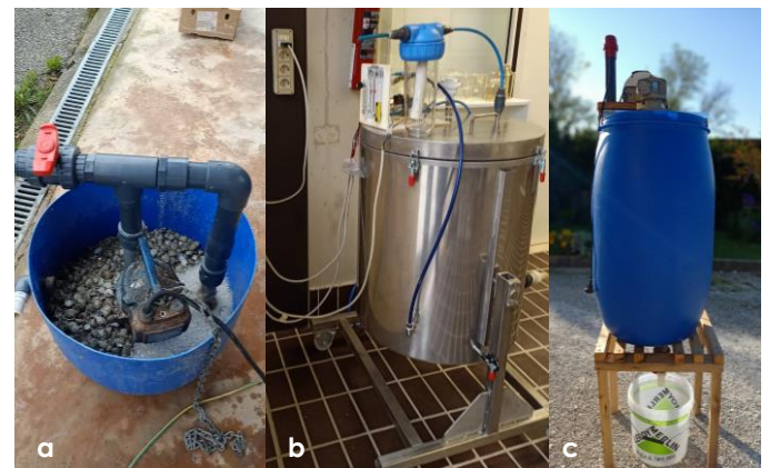
Fig 2: Shredding (a), composting (b) and hydrolysis (c) reactor
